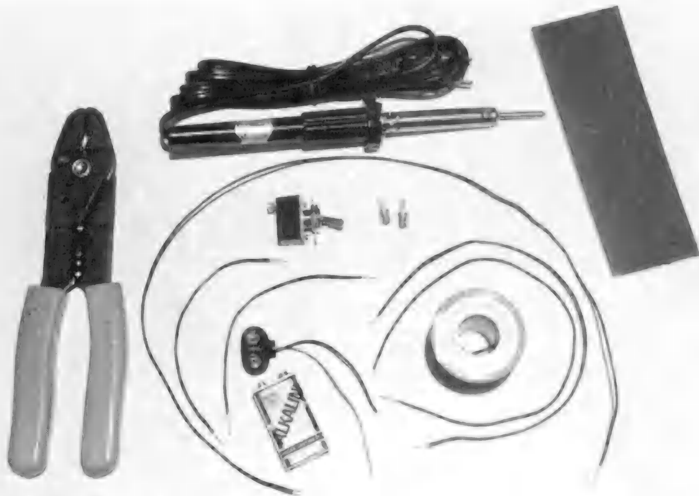
Everything you need to do the "glowing eyes" project is shown here. Note that a 9-volt battery clip has been added to make replacing the battery easier. All parts are available at Radio Shack stores.
